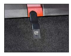
**STEP 12**Using the supplied 3/8-16 x 1-1/4" Hex Head Bolt, install the Top Center Bracket as shown.
